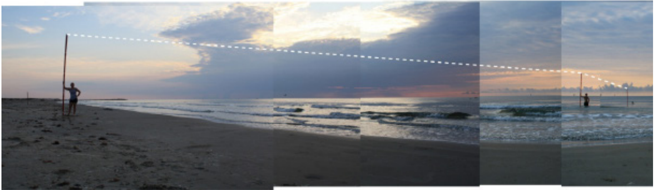
Figure 3. The simple tool, an oversized measuring stick, provided a constant within a series landscape photographs and increased their capability to measure during the extended site visit. Image credit: Jeff Carney.
